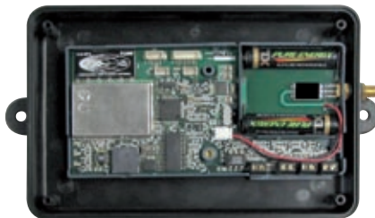
▲ Wireless power charges the batteries in a zoo's temperature sensors. An antenna (not shown) picks up an RF signal and feeds it to the Powerharvester chip (between the batteries)
