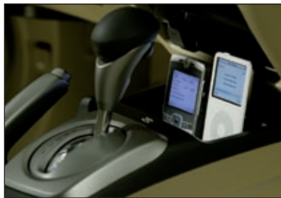
▲ eCoupled works over a very short range, but caddies and mats built into furniture or cars will charge any device placed on them
