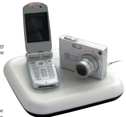
▲ Induction mats can transfer power to compatible devices wirelessly
